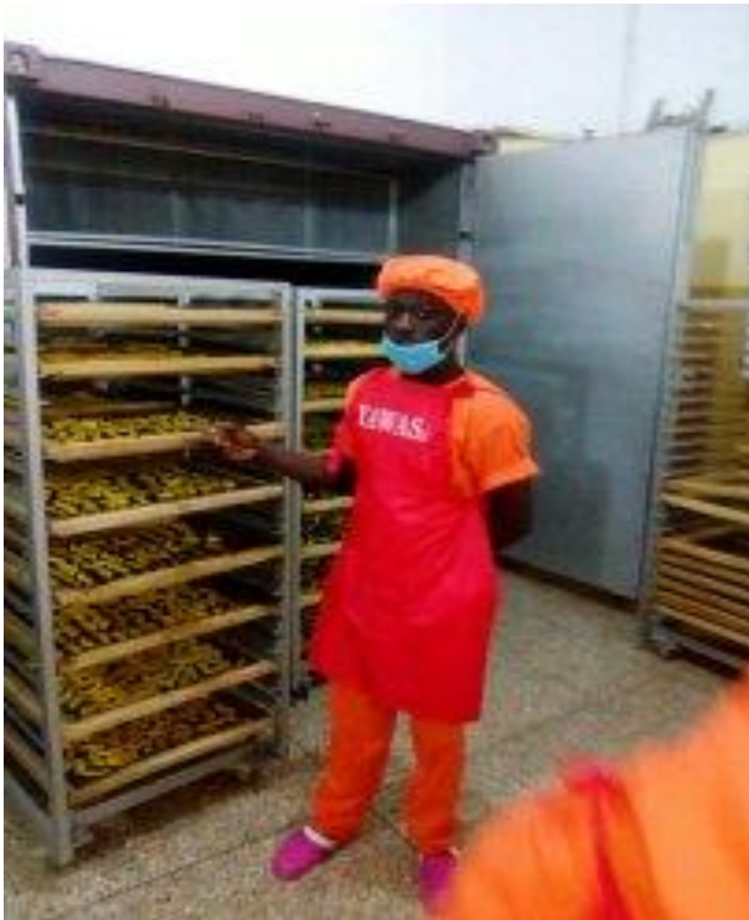
Figure 24: AFTER 11 HOURS OF DRYING BETWEEN 65-70 DEGREES, CHECK MOISTURE BY FEELING/TASTING. WHEN IT IS RIGHT REMOVE TROLLEYS FROM OVEN AND POSITION THEM TO A COOLING AREA
