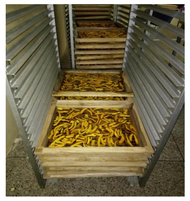
Movable trolleys with wheels are used to load fresh sliced mangoes. There are 12 trolleys that are filled with 30 trays. Immediately the trolleys are full they are sent into the oven to prevent contamination.
