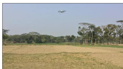
Use of Octocopter to capture multi-spectral images
