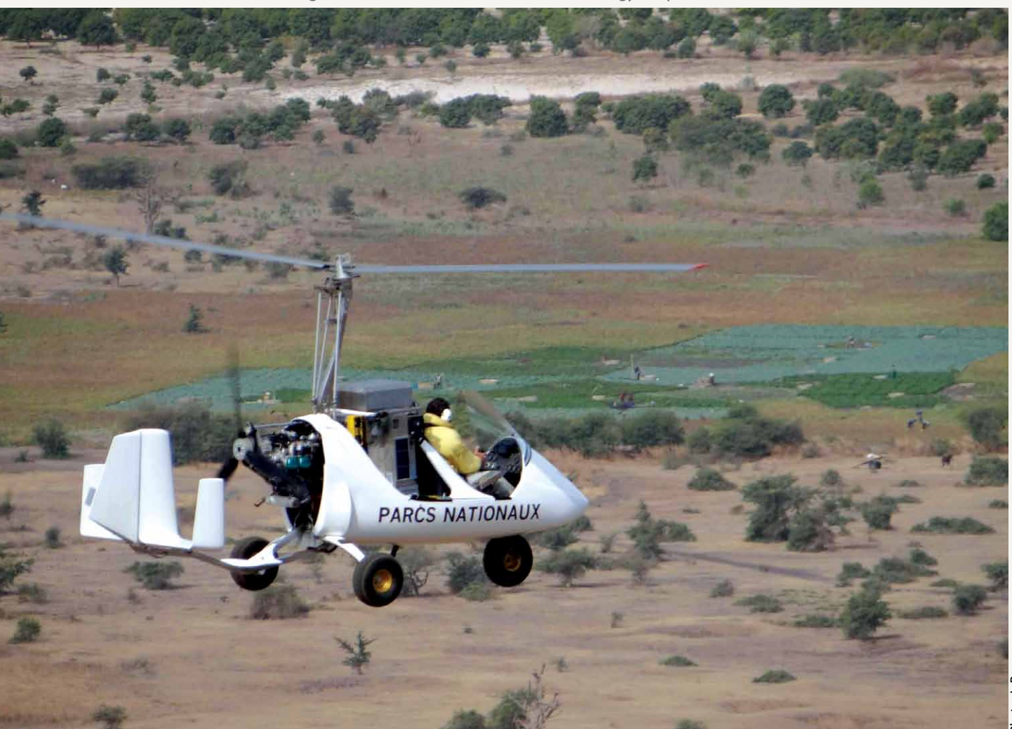
Release of sterile males using an automatic release machine on board a gyrocopter
